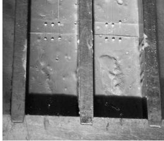
Fig. 5: EFPI sensors during embedment into cement paste (bodies: 4 cm x 4 cm x 16 cm).
