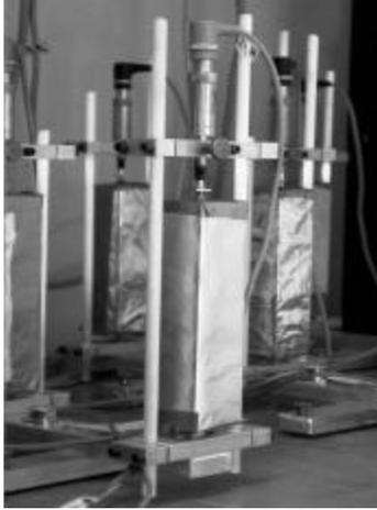
Fig. 4: Cement paste specimens fixed in the frame and equipped with inductive displacement transducers.
