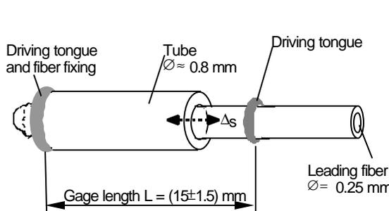
Fig. 2: Principle of compliant EPFI-sensor.
