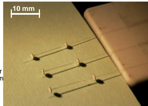
Fig. 3: Flexible EFPI sensors (fiber microdistometer) prepared for embedment (the driving tongues are designed as disks).
