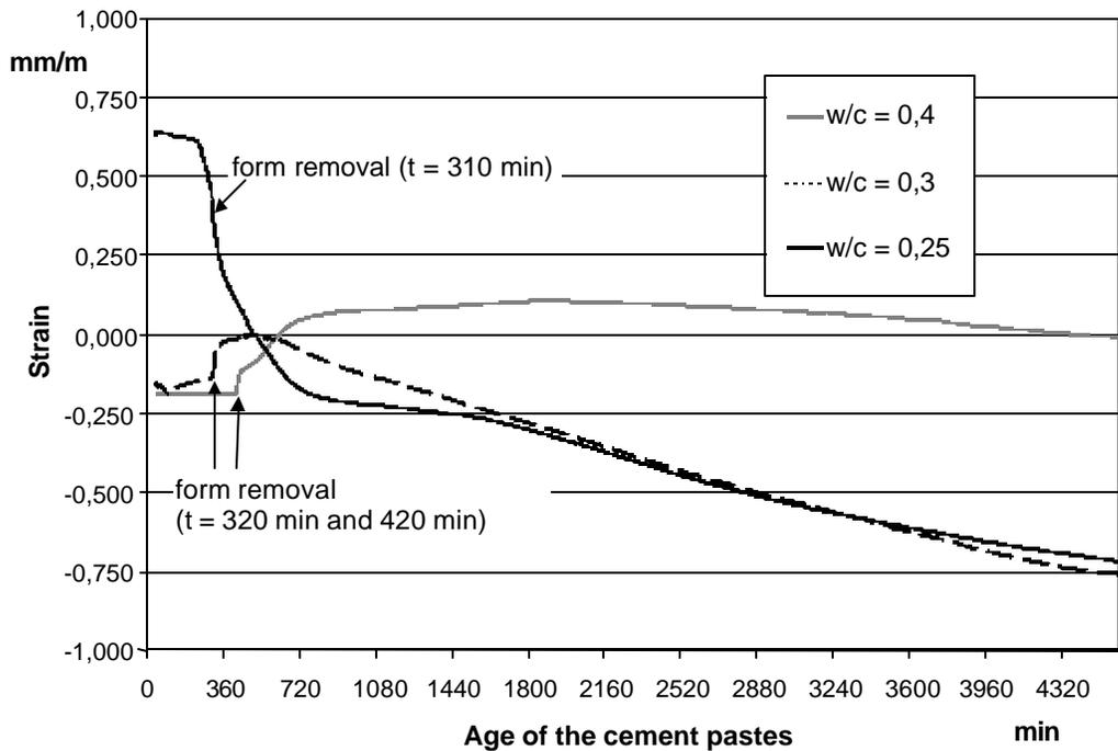
Fig. 7: Influence of water-cement ratio on deformation of Portland-cement paste (CEM I 42,5 R-NA) at early ages (in comparison with fig. 6),
