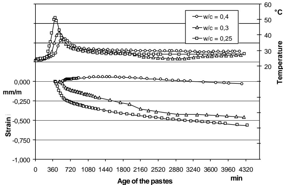
Fig. 6: Length changes of cement paste specimens depending on the w/c ratio uniaxially measured in the frame, temperature measured in the core of the specimen. (The length changes show temperature-influenced deformations).
