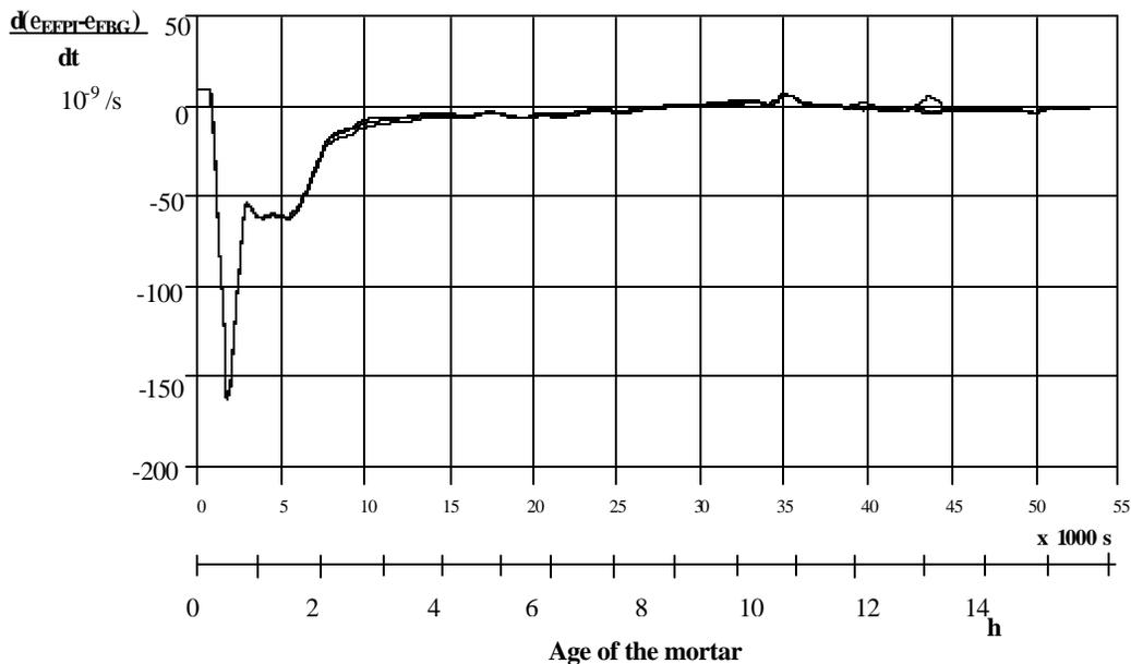
Fig. 1: Velocity of alignment of the matrix deformation measured by stiff Bragg grating sensors with those measured by compliant (EFPI) fiber sensors (beam: 80cmx8cmx4cm).
