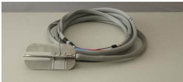
Figure 3: Probe with Guide Vanes Connected (Up Gas Flow Velocity Scenario)
