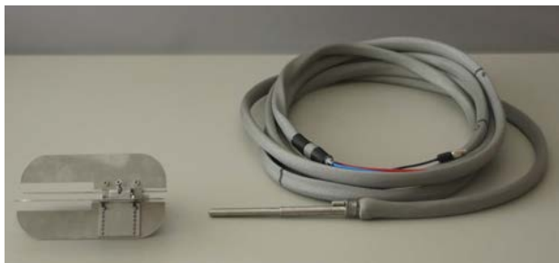
Figure 2: Probe with Guide Vanes Disconnected (Pulse Pressure Peak Scenario)
